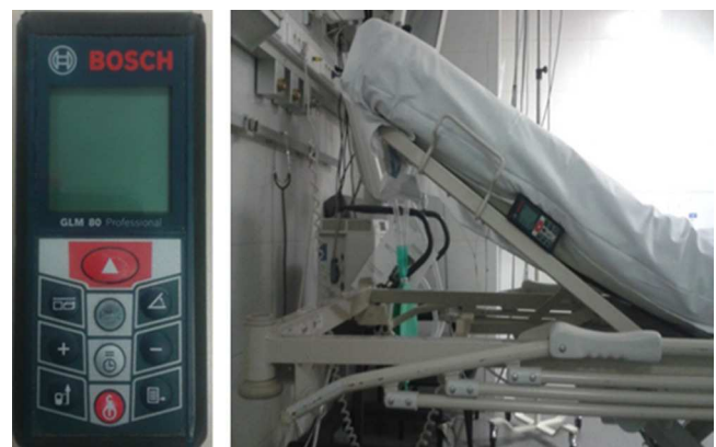
Figure 1 Device used for the measurement of the head-of-bed elevation and technique for the measurement of the backrest elevation (Bosch® GLM 80).
