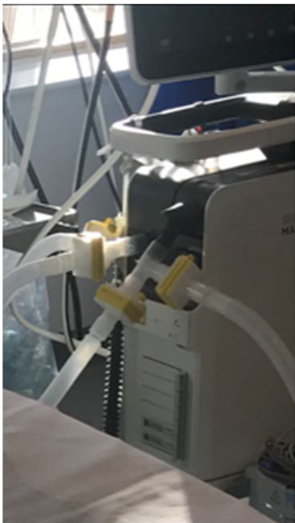
Figure 1 Two sets of standard ventilator tubing (Hudson) were connected to a single ventilator (tested in each model of ventilator, Puritan-Bennett, 840 series and a Servo I Maquet) via two T-tubes (one on the patient inflow limb of the circuit, and one on the patient exhaust limb). Each T-tube was attached to a microfilter (total of four) to isolated both patients and the ventilator. Especially if the circuit do not have in place non-return valves.
