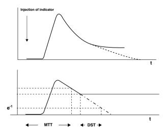
**Figure 1** The upper curve indicates a thermodilution curve obtained by injection of a cold bolus, showing the temperature over time at the catheter tip. By extrapolation of the curve (dashed line), potential recirculation phenomena are excluded. The lower curve shows the logarithmic extrapolation allowing to define the mean transit time (MTT) and the exponential downslope time (DST) of the indicator.
