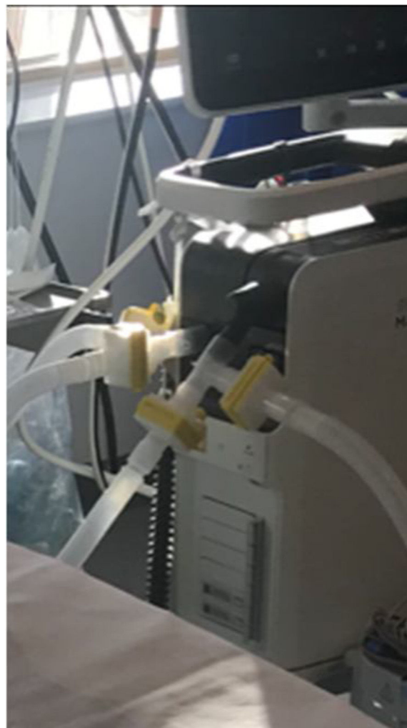
Figure 1 Two sets of standard ventilator tubing (Hudson) were connected to a single ventilator (tested in each model of ventilator, Puritan-Bennett, 840 series and a Servo I Maquet) via two T-tubes (one on the patient inflow limb of the circuit, and one on the patient exhaust limb). Each T-tube was attached to a microfilter (total of four) to isolate both patients and the ventilator. Especially if the circuit do not have in place non-return valves.
